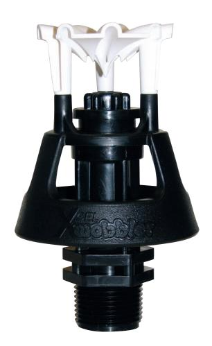
Senninger's Xcel-Wobbler is ideal for reducing over watering by allowing wide spacing (up to 20 feet) and providing a wind-resistant pattern with extremely uniform coverage. The Xcel-Wobbler is a low pressure 10 psi sprinkler that is mounted on the top of the pipe along the first two spans of a center pivot or other mechanical-move system.
