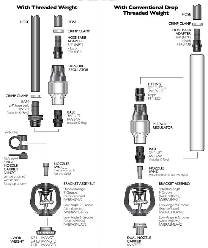
Note: Selection of weight style (location) is based on application and preference. Only one style weight should be used per i-Wob.
