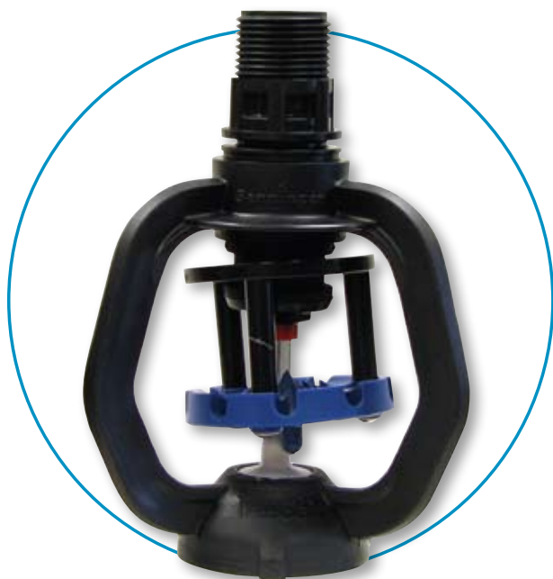
Low-Angle: 9-Groove blue deflector, smaller droplets
